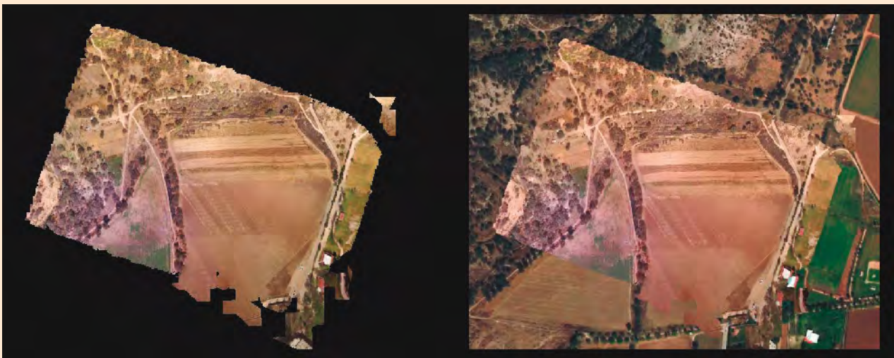
Validation of orthophoto. The output image obtained by ODM is show on the left. To the right, this output ( the geo-referenced tif image) is mounted on a web mapping software.
